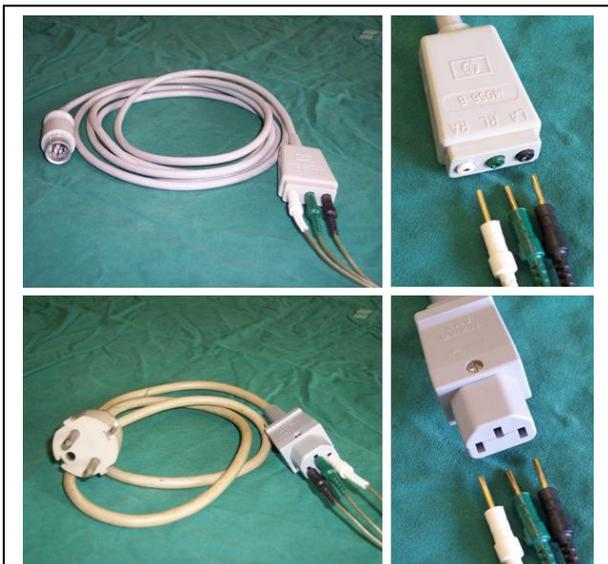
Fig. 1: Murphy's Law illustrated. 2mm male pins of old-style ECG-electrode lead wires normally plug into an ECG patient cable (both upper photos). These pins also fit into worldwide used female IEC mains plug (both lower photos).
