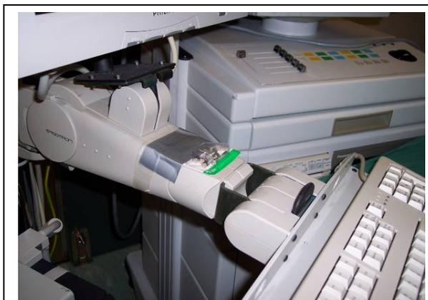
Fig. 2: Example of "tape analysis". Shown is an OEM supplied trolley, which by itself fulfilled all requirements of IEC 60601. Violating this standard, the trolley was retrofitted with equipment drawing more power than the built-in safety transformer was specified for. Therefore the built-in fuses sometimes blew. Following the principle of Le Châtelier & Van't Hoff, someone "solved" the problem by taping spare fuses to the keyboard support arm (see middle of photo).
